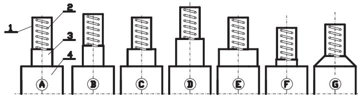
Fig. 4. Configuration of different combustion chambers in relation to prechamber and engine cylinder (in scale): 1 – prechamber, 2 – catalytic wire, 3 – combustion chamber, 4 – engine cylinder. Letters in a circle indicate the notation shown in Table 2
