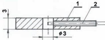
Fig. 2. Outline of the combustion chamber (type B in Table 2) together with the temperature probe: 1 – combustion chamber, 2 – temperature probe
