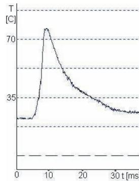
Fig. 3. Temperature inside the combustion chamber during compression process
