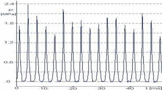
Fig. 8. Cylinder pressure as a function of time for model engine
